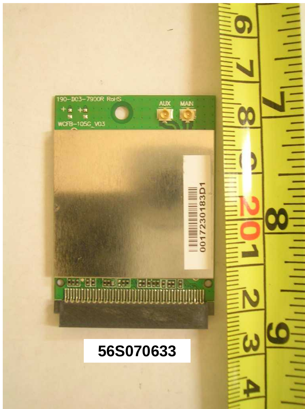
WLAN 802.11b/g Module Board PCB Component Side
