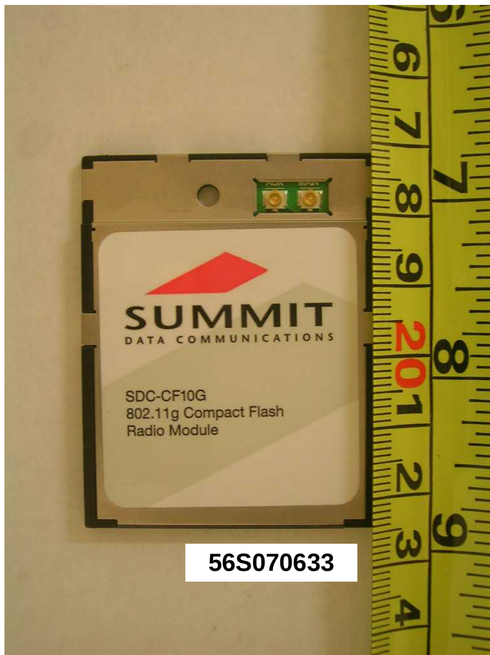
WLAN 802.11b/g Module - Front View
