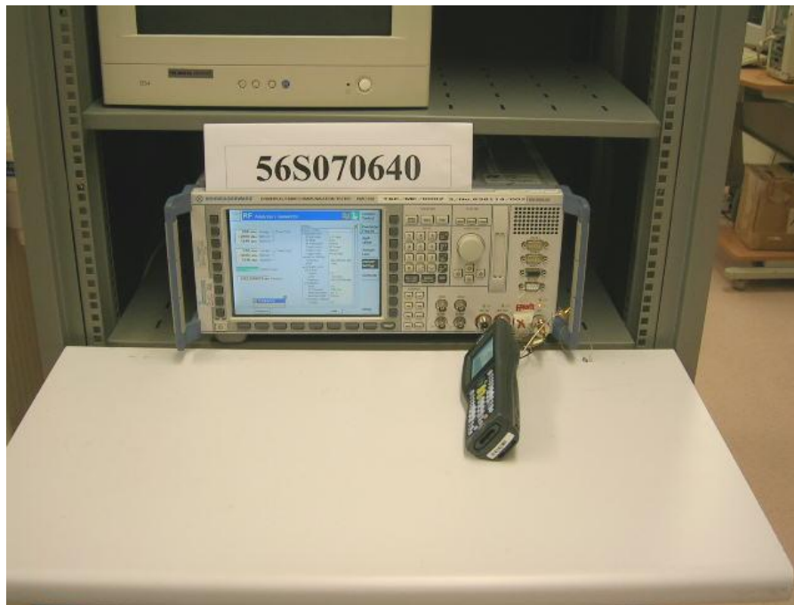
Conducted Power Measurement Setup
