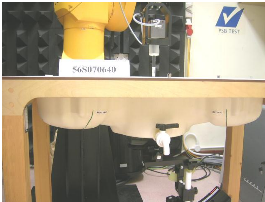
SAR Test Setup (Device at Body phantom)
