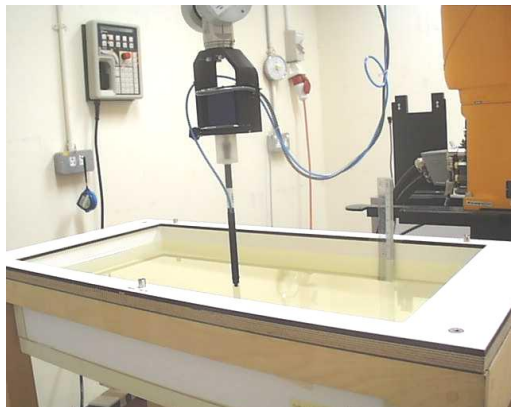
At “450MHz Flat Phantom – 2mm Shell Thickness”
