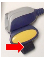
Figure 8 Concept - Ring Scanner Hook and Loop Strap
