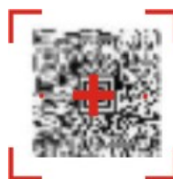
Figure 27 Imager Bracketed Crosshair Target on 2D Barcode
