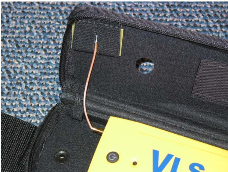
Antenna Mount in Unit
