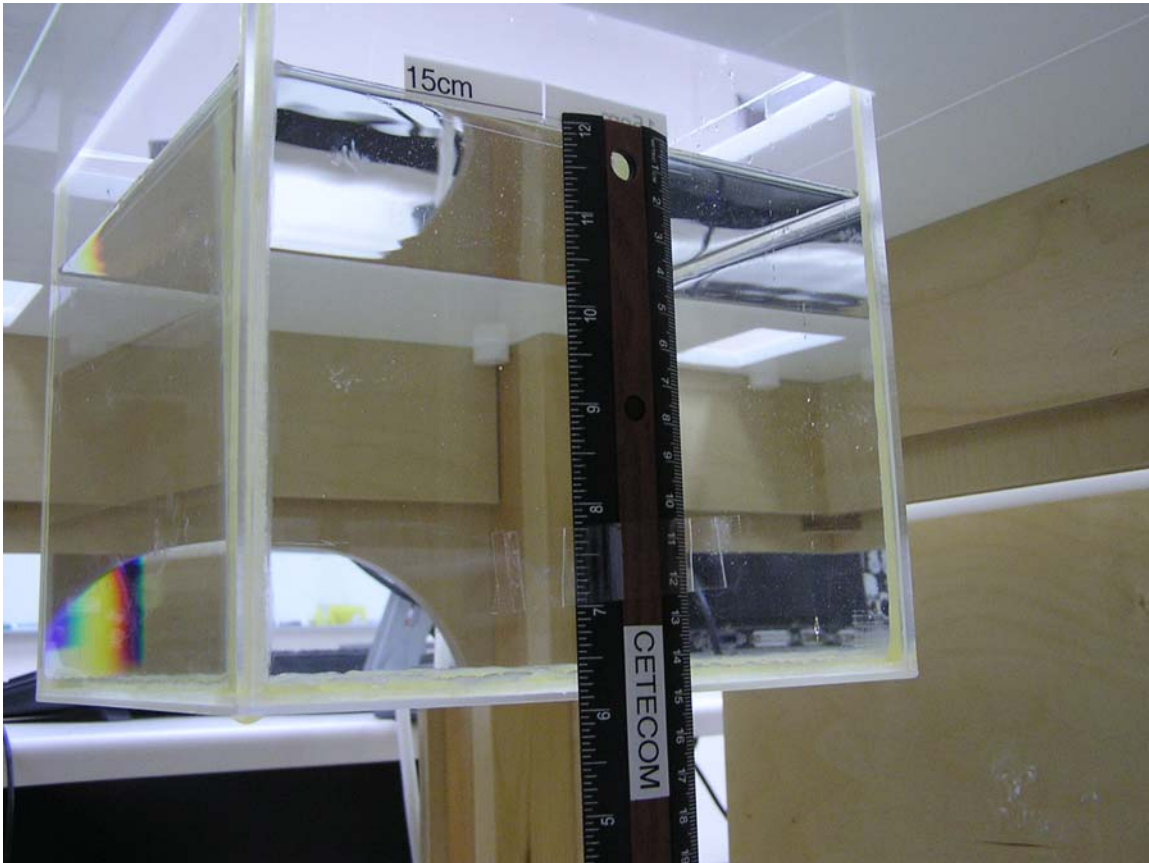
Photo 5. Photo to demonstrate 15 cm Z-axis flat phantom
