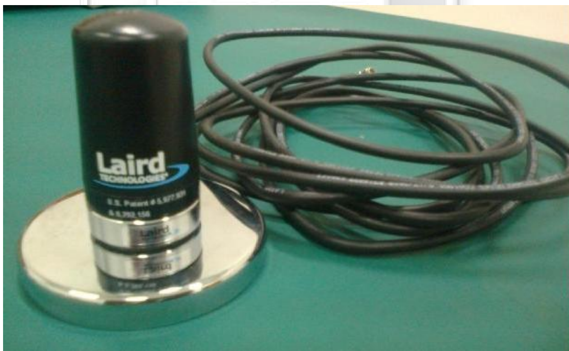
Mobile Net Antenna : Laird (Type : Multi Band Phantom, Type : Trab806/17103 & Miniature Magnetic Mounts, Type : G16404 Attached With Attached 12ft Cable)
