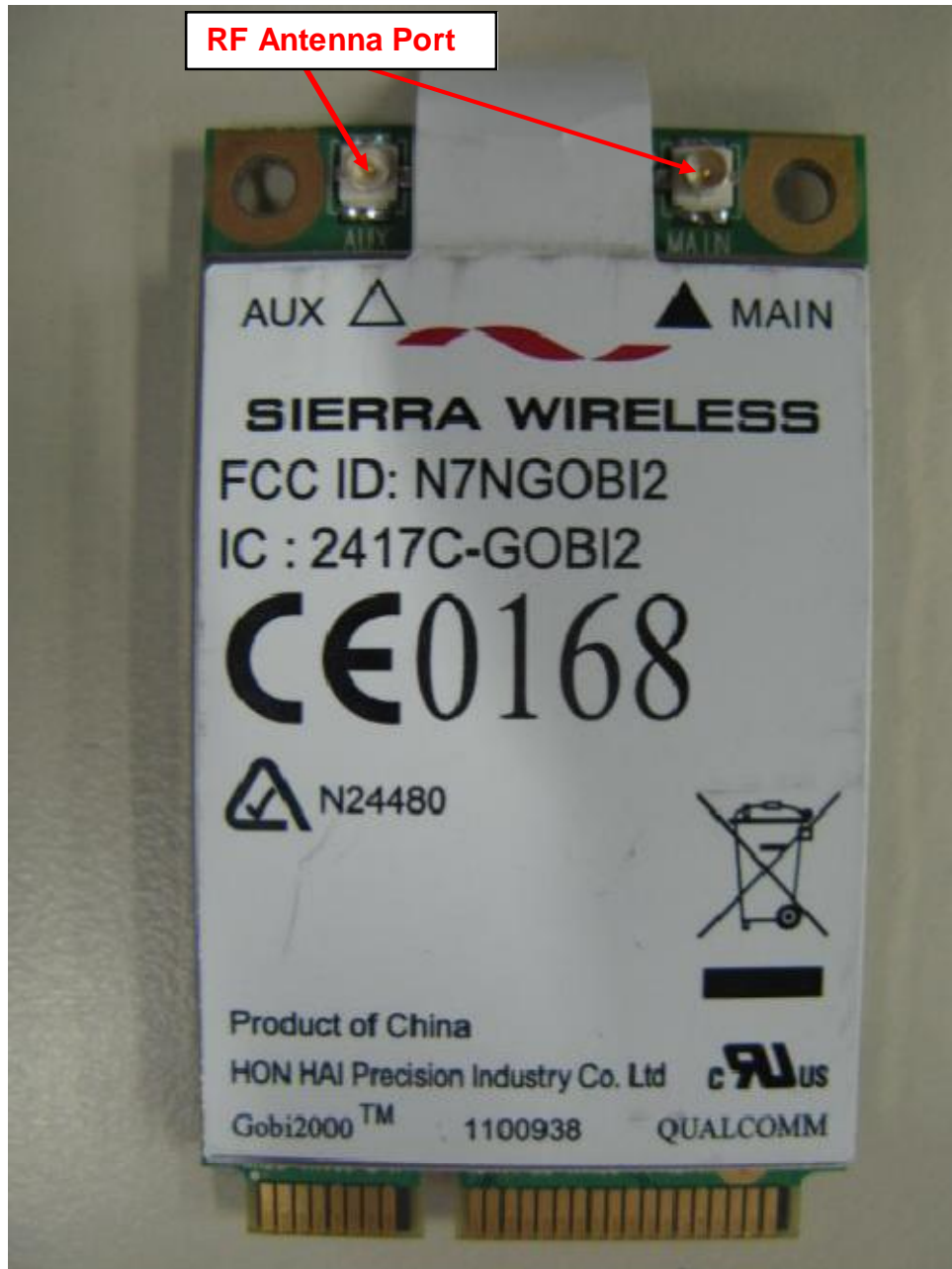
WWAN Module PCB Component Side
