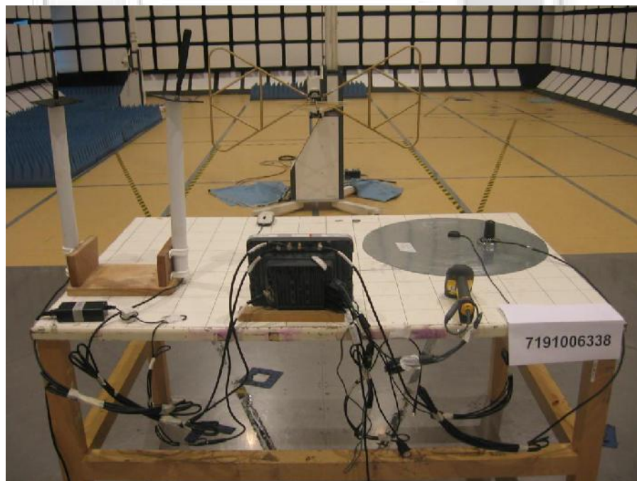
Radiated Emissions Test Setup (Rear View)
