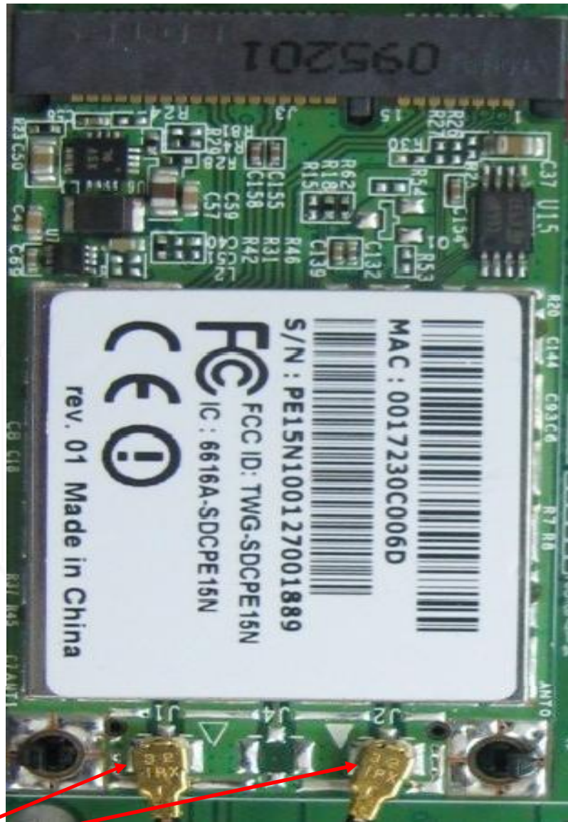
WLAN Module-PE15N PCB Component Side
