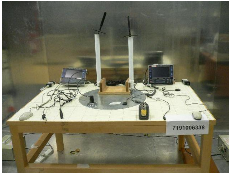
Conducted Emissions Test Setup (Front View)
