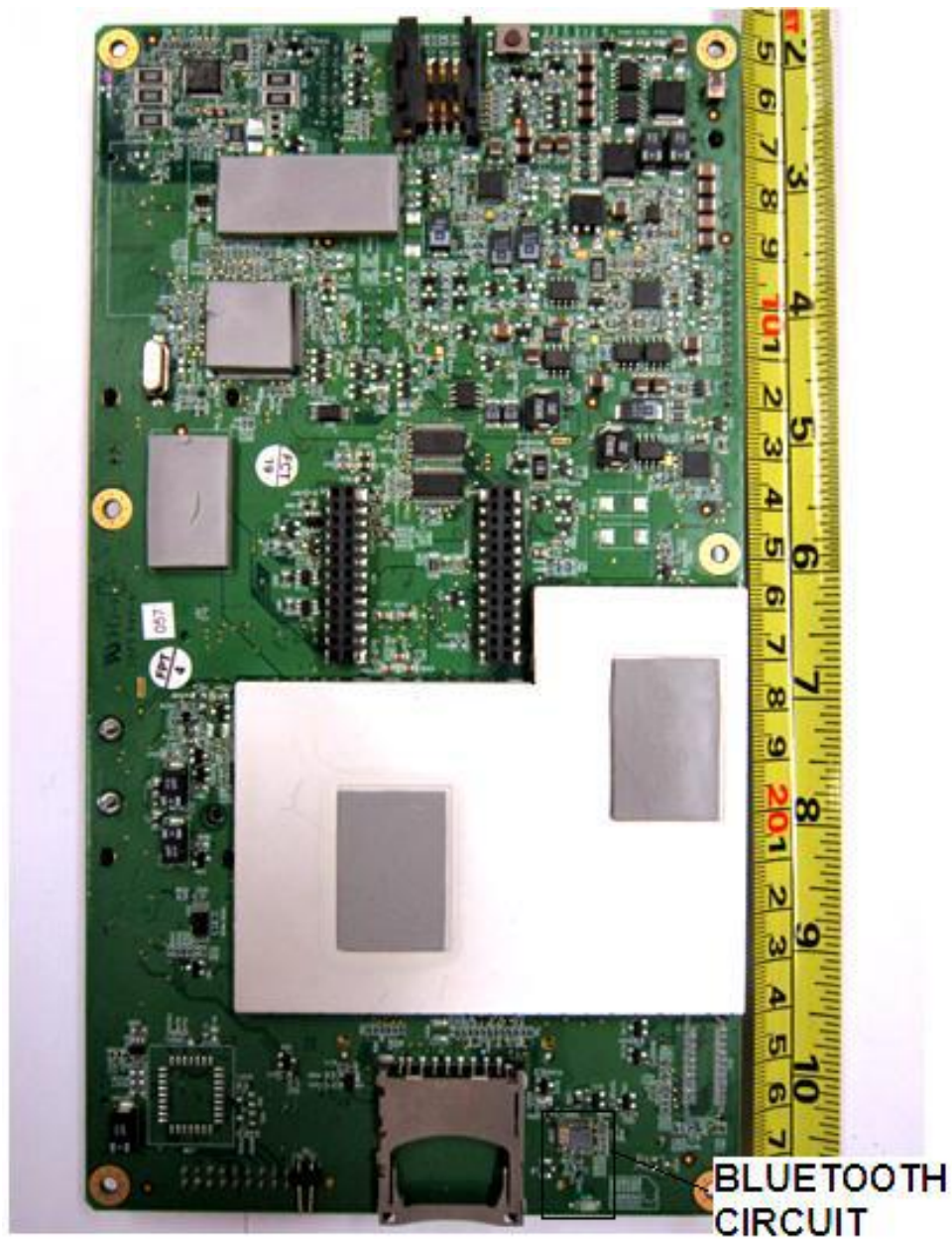
Bluetooth-Module PCB Component Side
