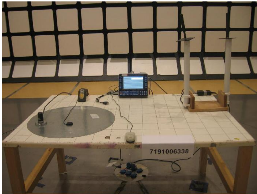
Radiated Emissions Test Setup (Front View)
