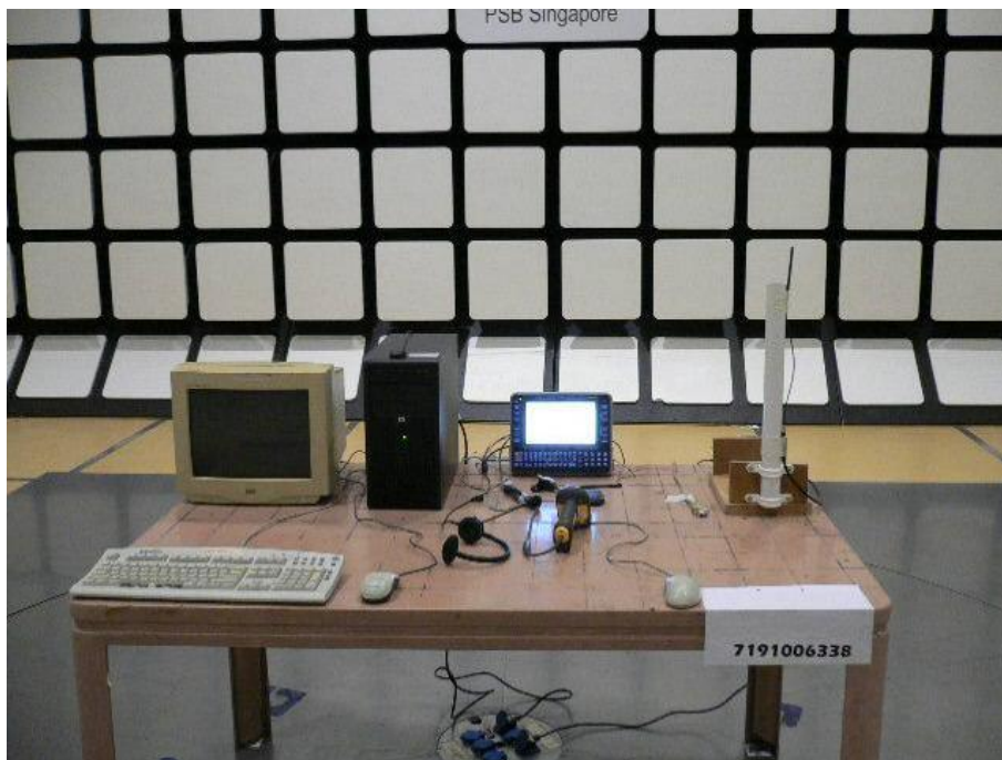
Band Edge Compliance (Radiated) Test Setup
