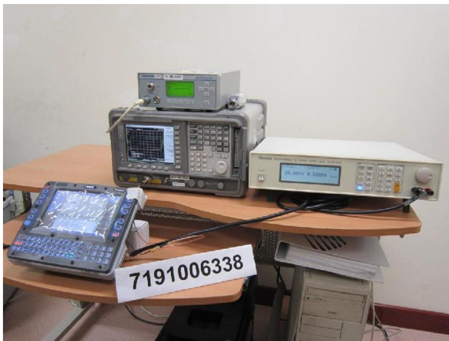
Peak Power Spectral Density Test Setup
