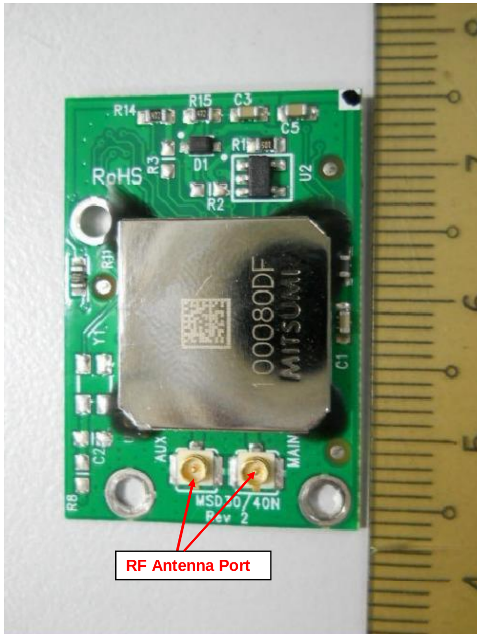
WLAN Module-MSD30AD PCB Component Side
