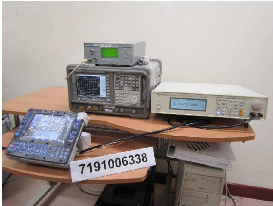
RF Conducted Spurious Emissions Test Setup
