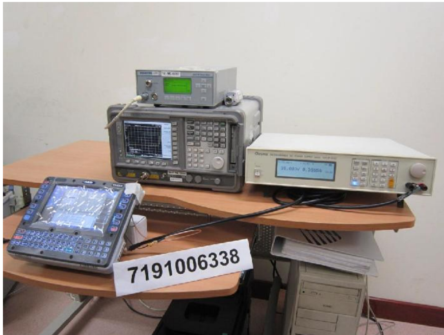
Number of Hopping Frequencies Test Setup
