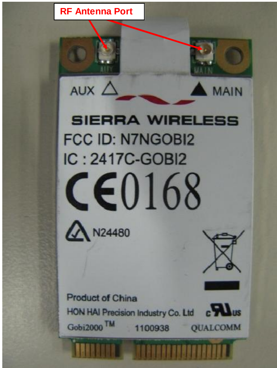
WWAN Module PCB Component Side
