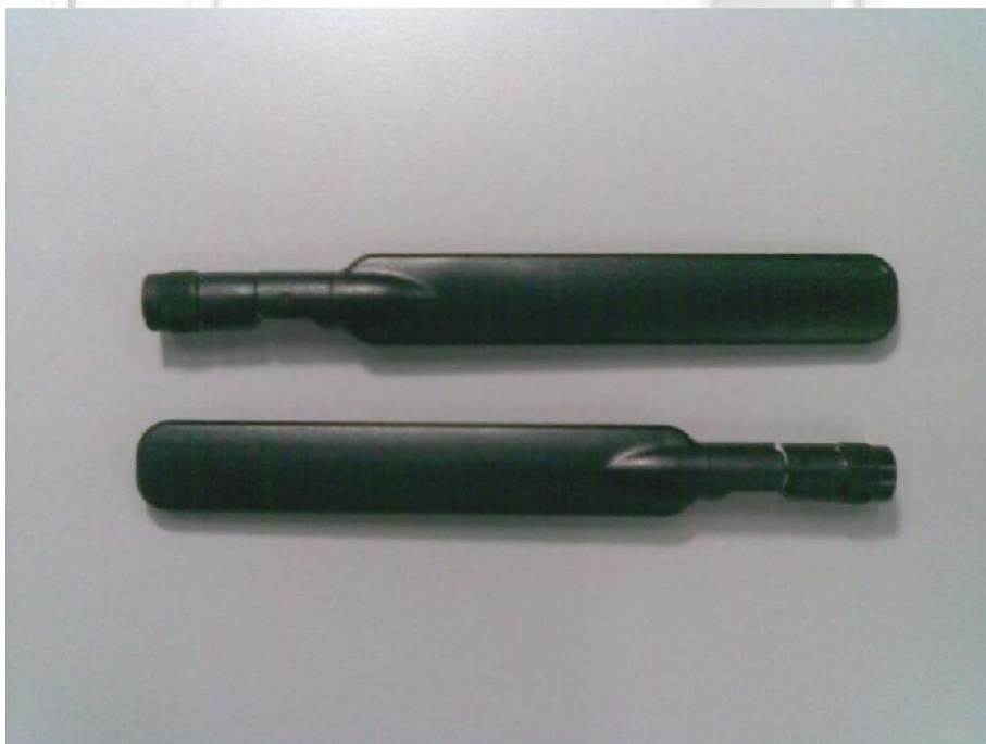
WLAN External Antennas : Larsen (Type : R380500314)
