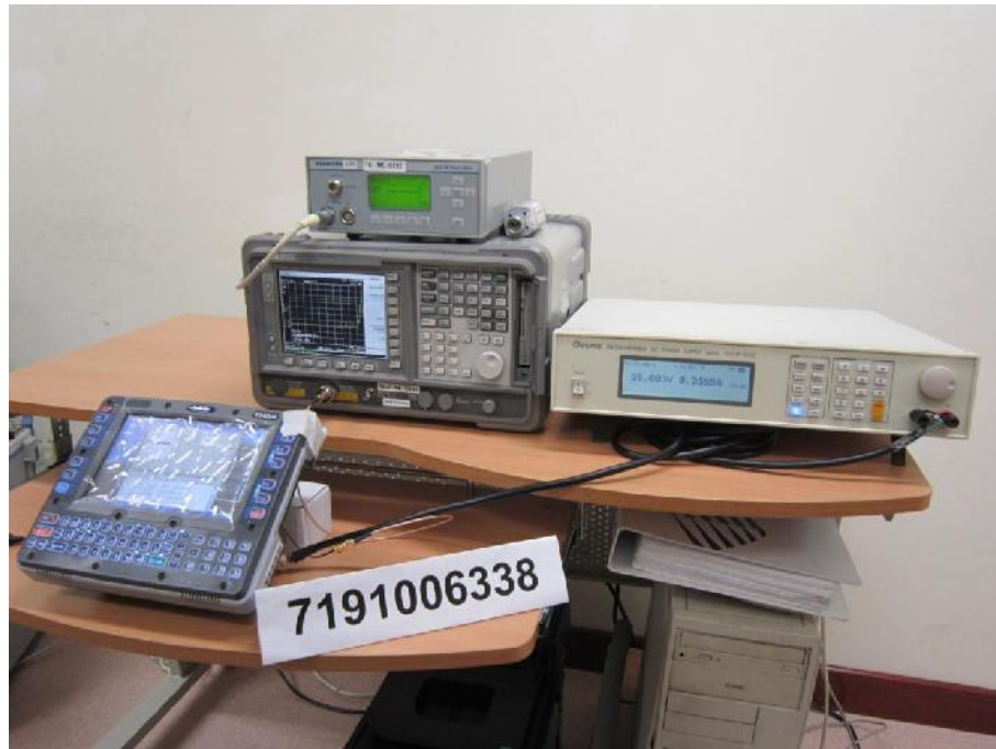
Average Frequency Dwell Time Test Setup
