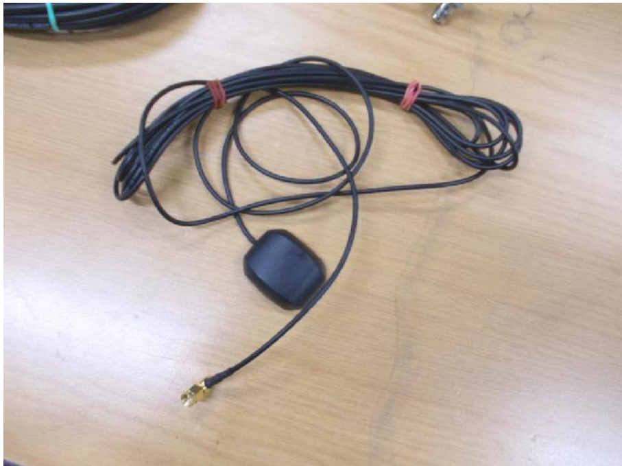
GPS Antenna : Laird (Type : GPS15MGSMB With Attached 4.8m RF Cable)
