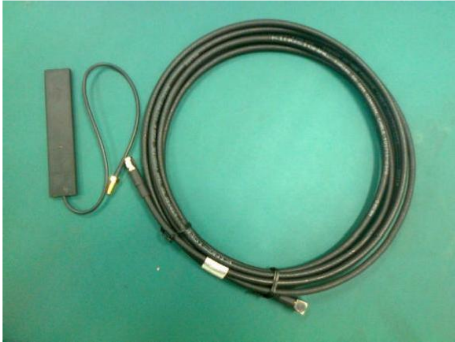
Mobile Net Antenna : Pulse (Type: W1923g0300) & Cable (Type: Rdn1007129)
