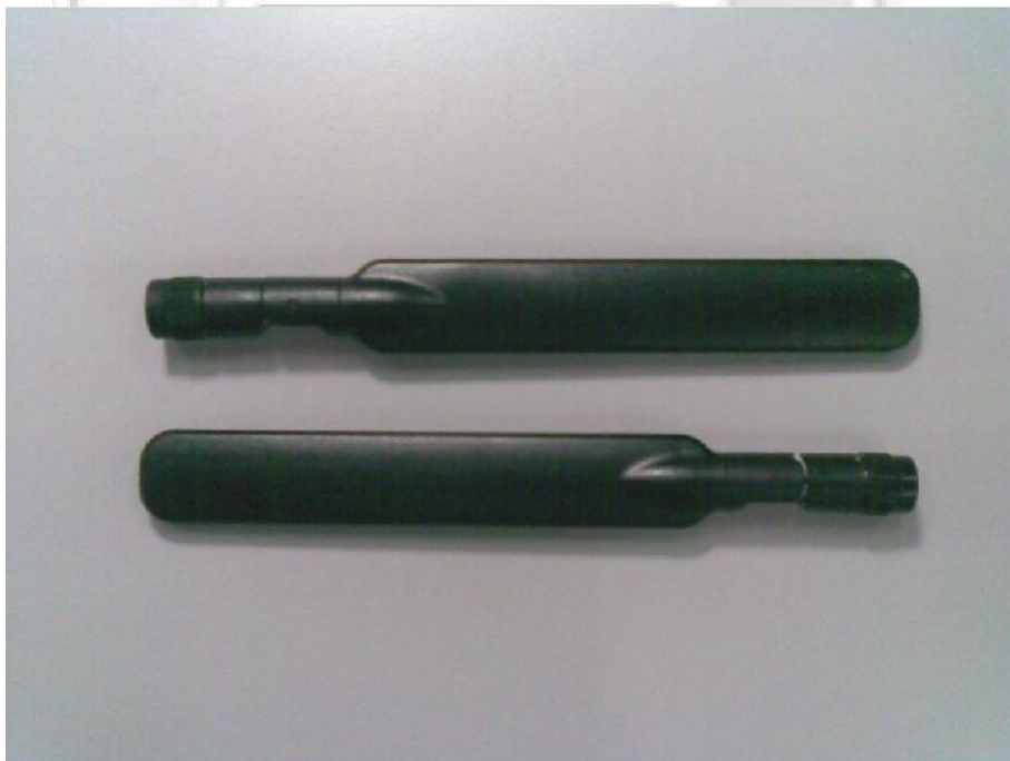
WLAN External Antennas : Larsen (Type : R380500314)
