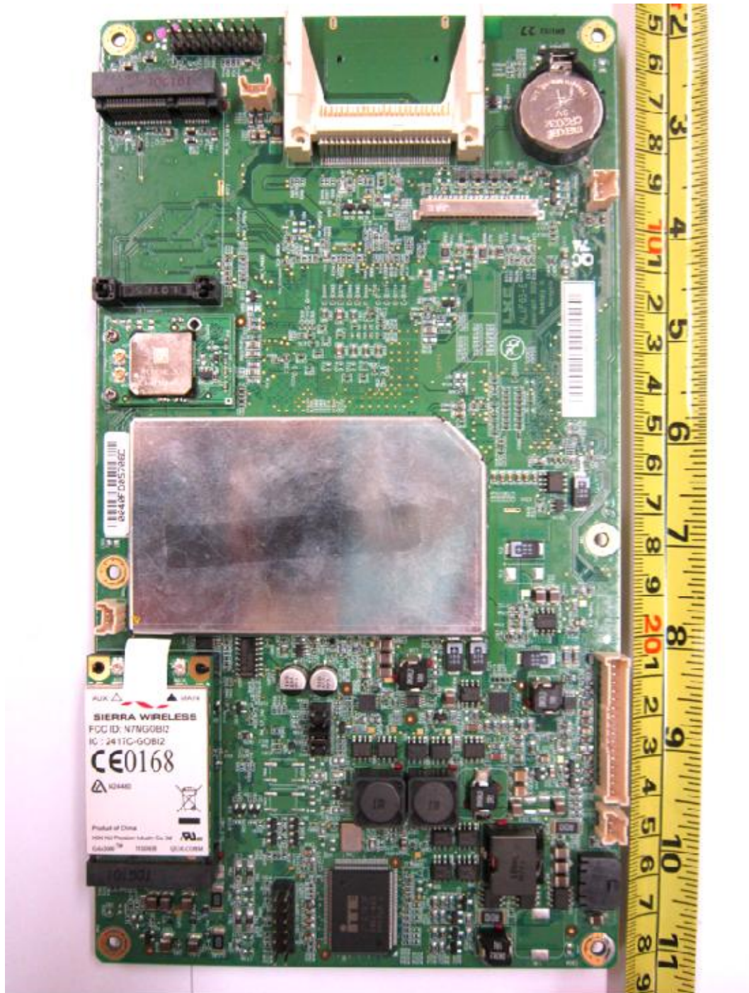
Main-Board PCB Component Side
