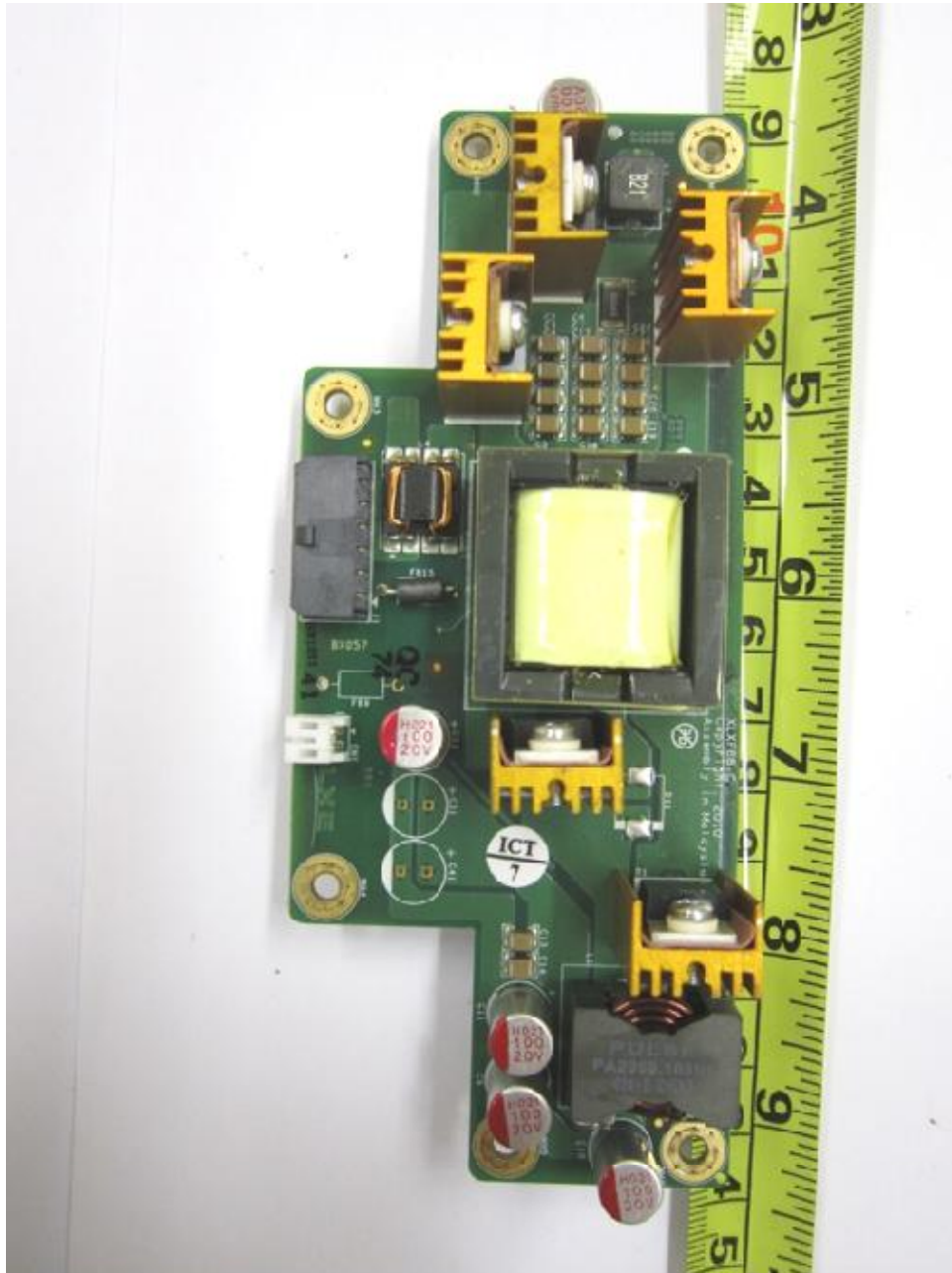
DC-DC Converter PCB Component Side
