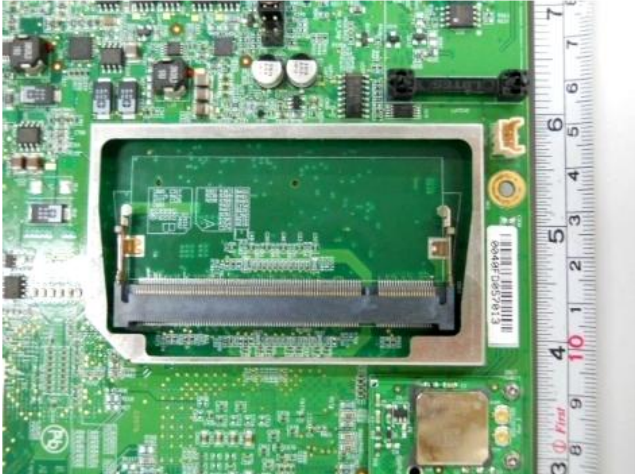
Memory DDR2-SDIO Shield Cover Removed Module PCB Component Side
