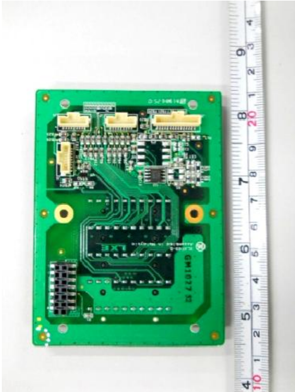
Docking Interface PCB Trace Side
