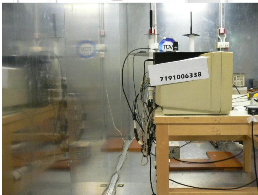
Conducted Emissions Test Setup (Rear View)
