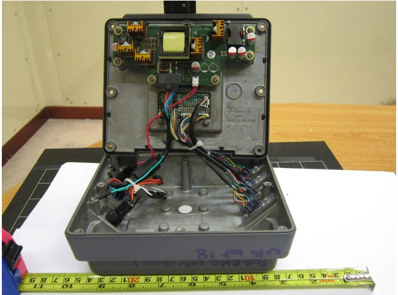
EUT Top & Bottom Housing Internal View
