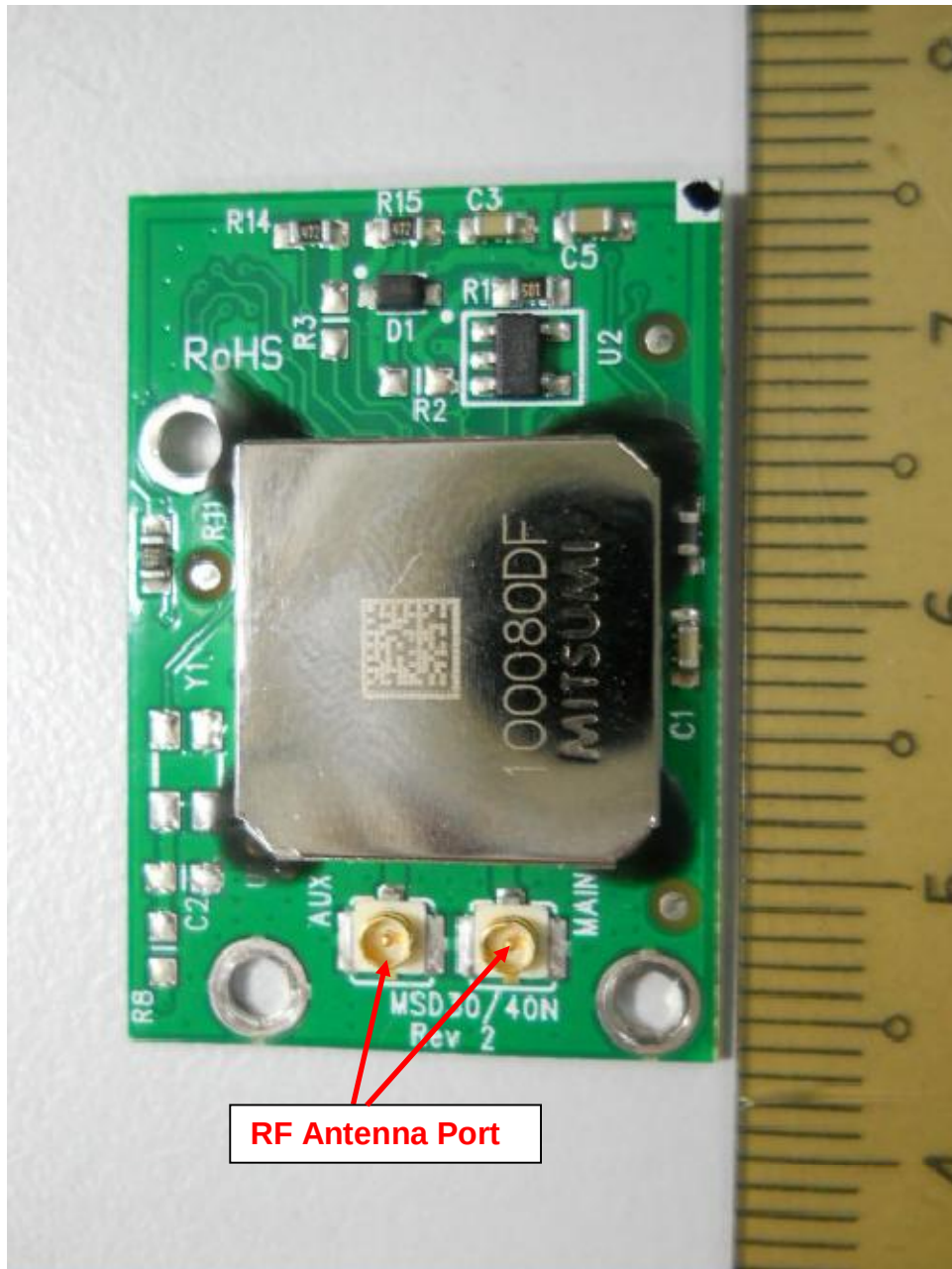
WLAN Module-MSD30AD PCB Component Side
