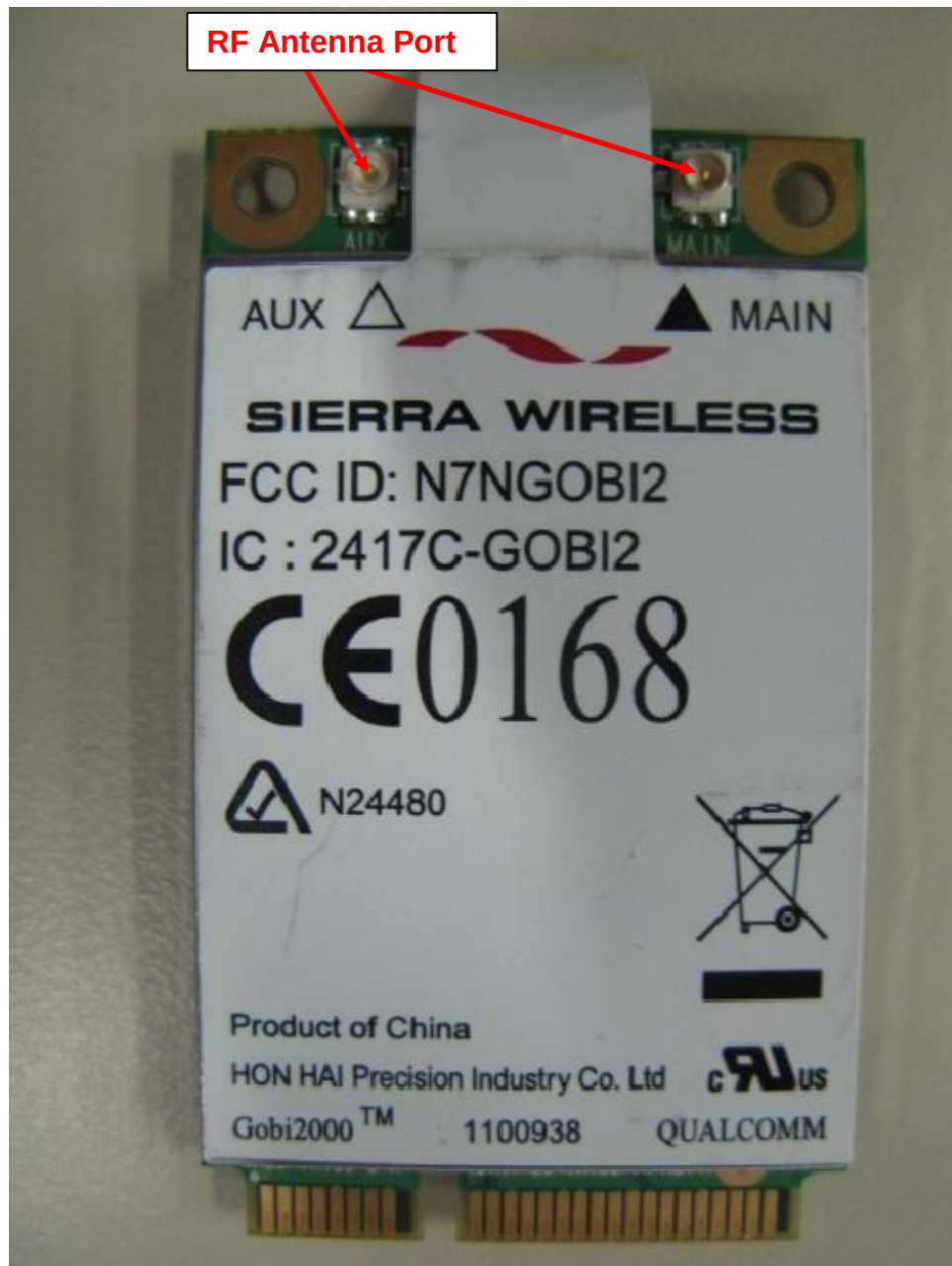
WWAN Module PCB Component Side
