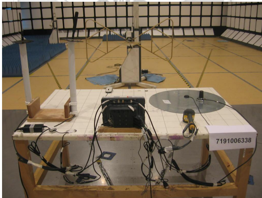
Radiated Emissions Test Setup (Rear View)
