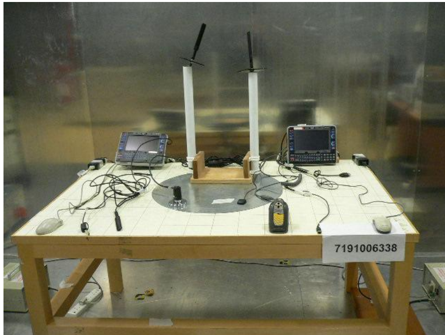
Conducted Emissions Test Setup (Front View)
