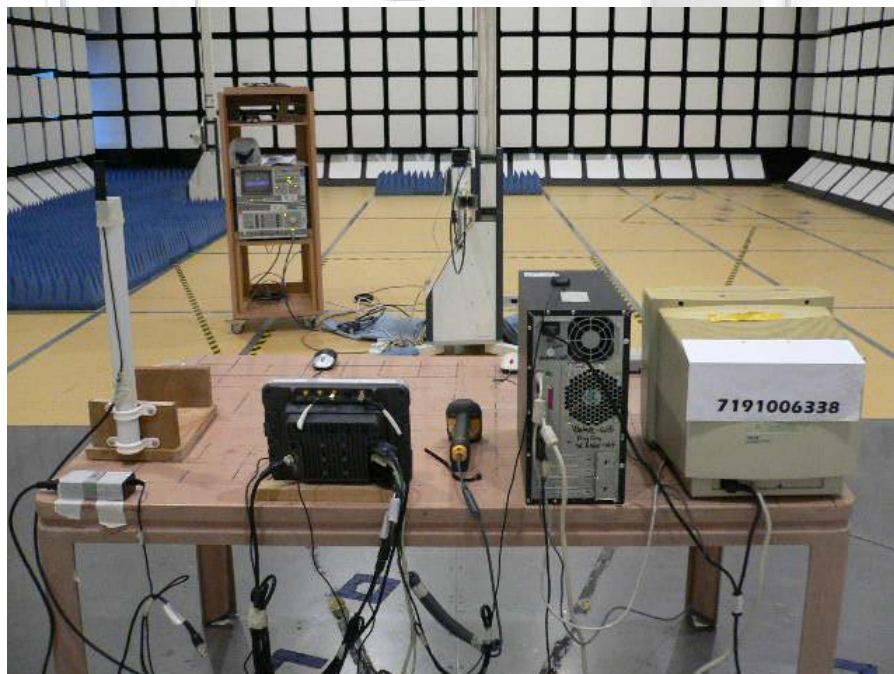
Radiated Emissions Test Setup (Rear View)
