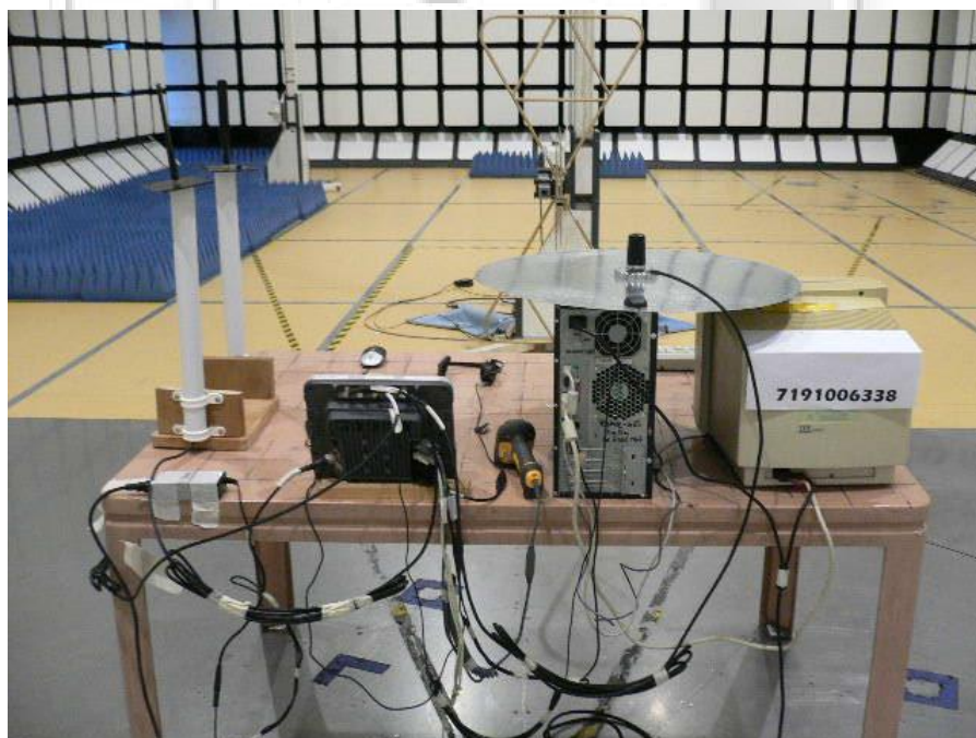
Radiated Emissions Test Setup (Rear View)
