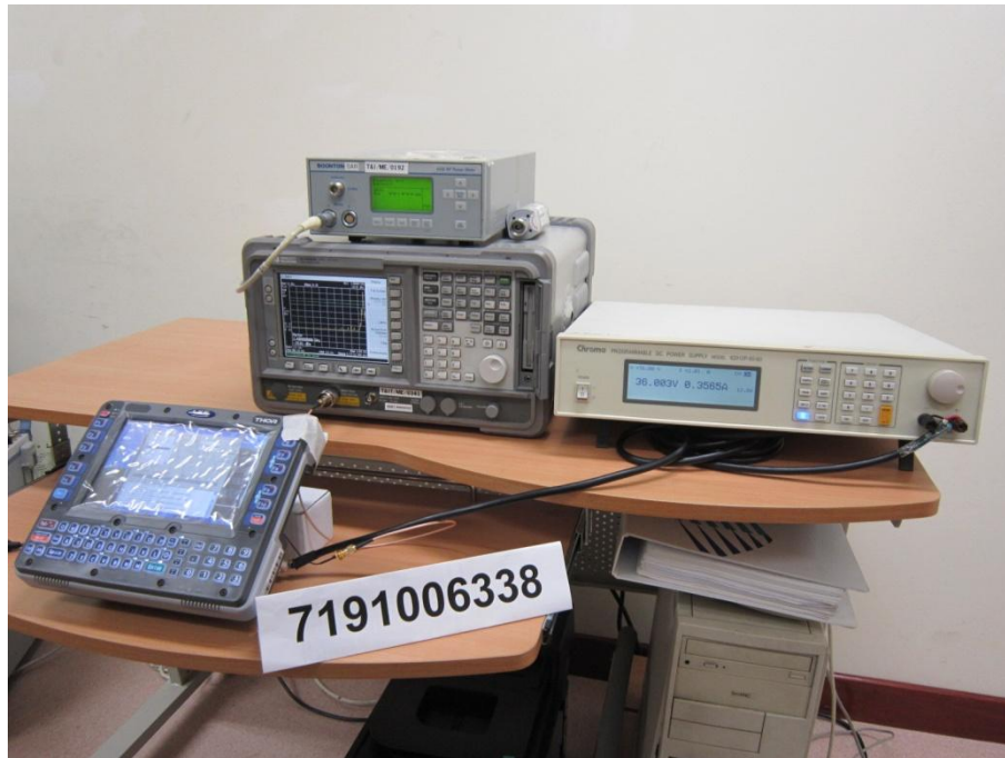
Average Frequency Dwell Time Test Setup
