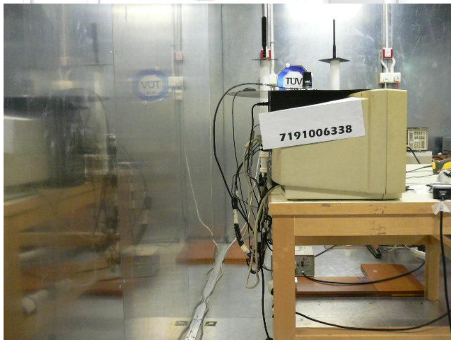
Conducted Emissions Test Setup (Rear View)
