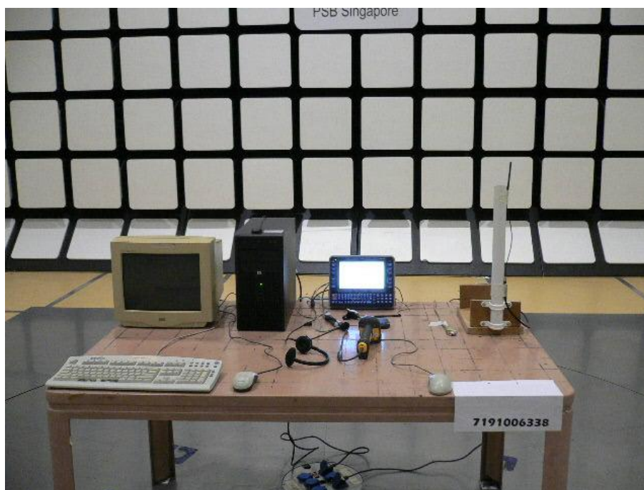
Band Edge Compliance (Radiated) Test Setup
