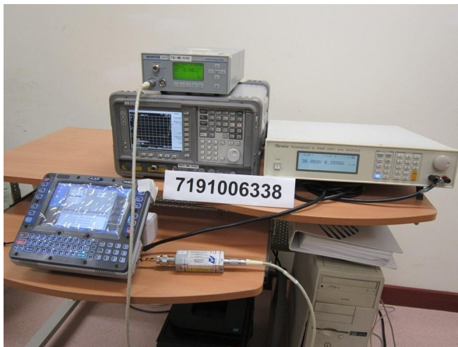
Maximum Peak Power Test Setup
