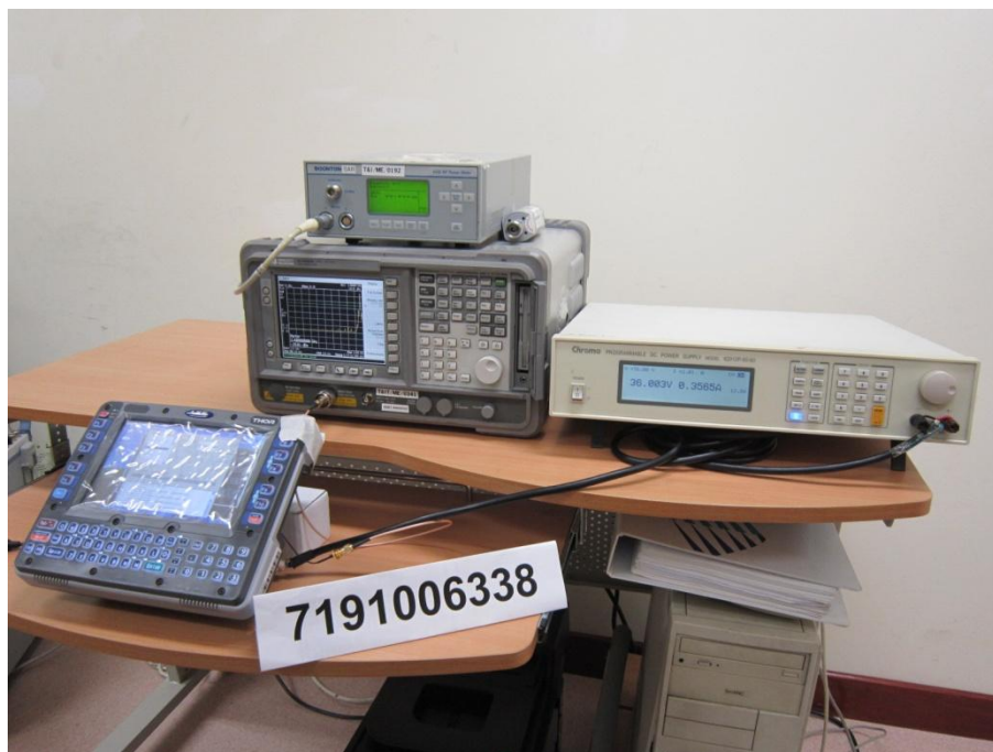
Carrier Frequency Separation Test Setup
