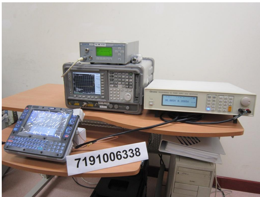
Band Edge Compliance (Conducted) Test Setup
