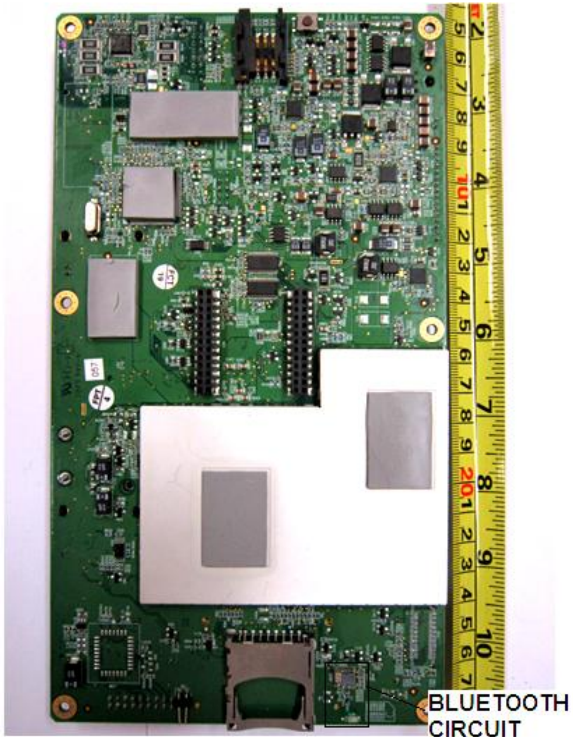
Bluetooth-Module PCB Location
