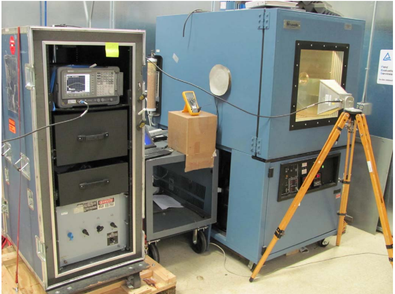
Figure 9 – View of EUT temperature Test Setup for Voltage Requirement tests..
