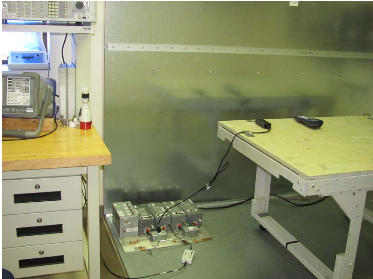
Figure 7: View of Conducted Emissions on AC Power Line test setup.
