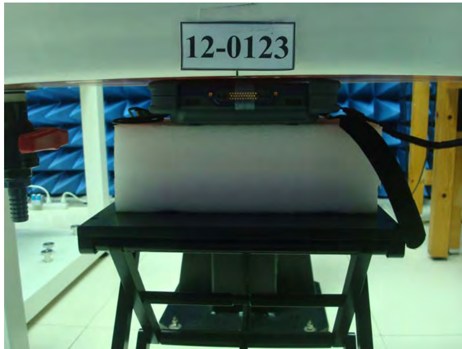
Body Setup (EUT with Hip Pad Battery and Hand strap, Front surface to phantom 0mm)
