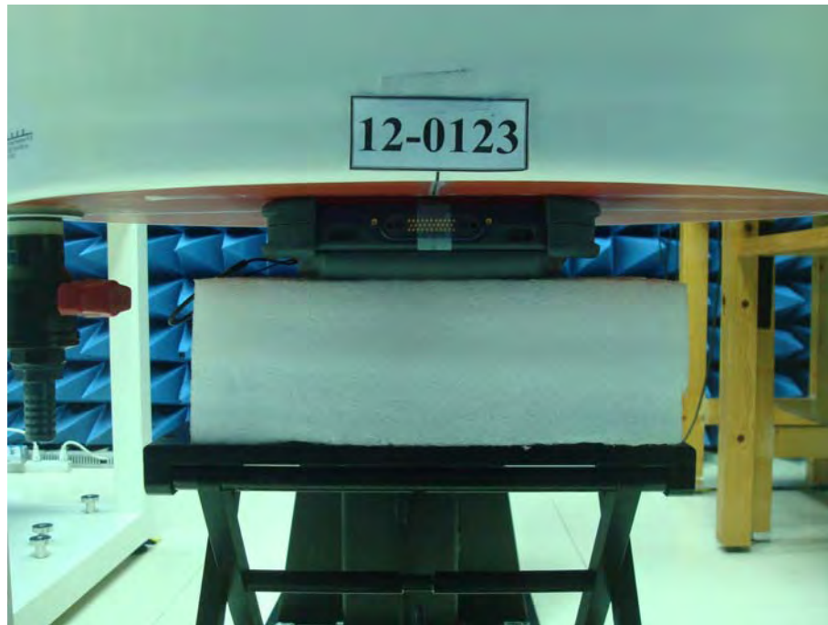
Body Setup (EUT with Hip Pad Battery, Front surface to phantom 0mm)
