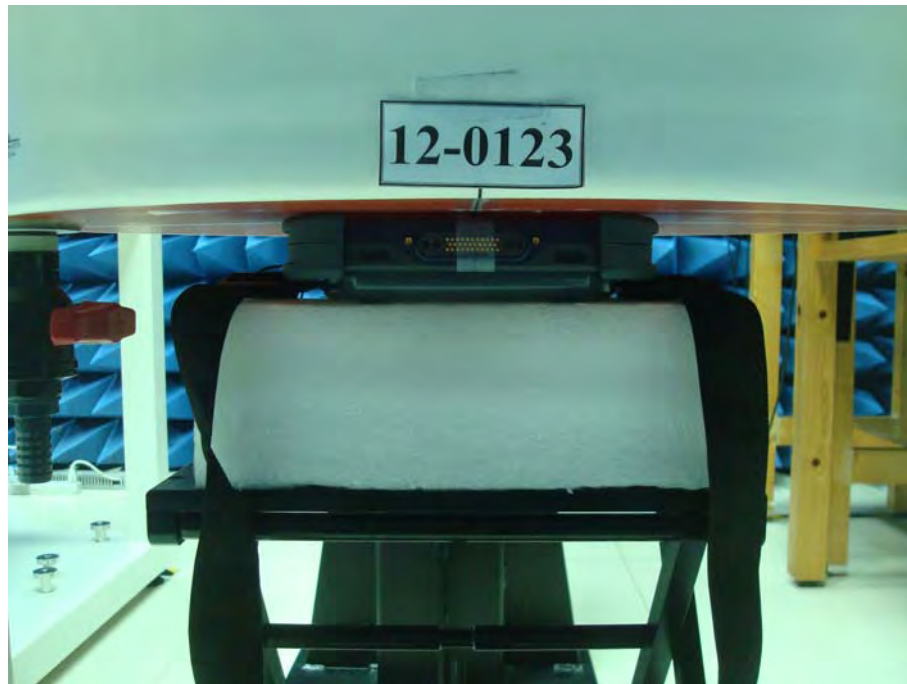
Body Setup (EUT with Thick Battery and Shoulder strap, Front surface to phantom 0mm)
