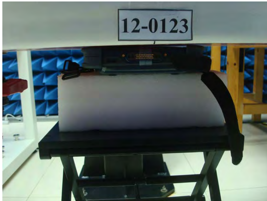
Body Setup (EUT with Thick Battery and Hand strap, Front surface to phantom 0mm)
