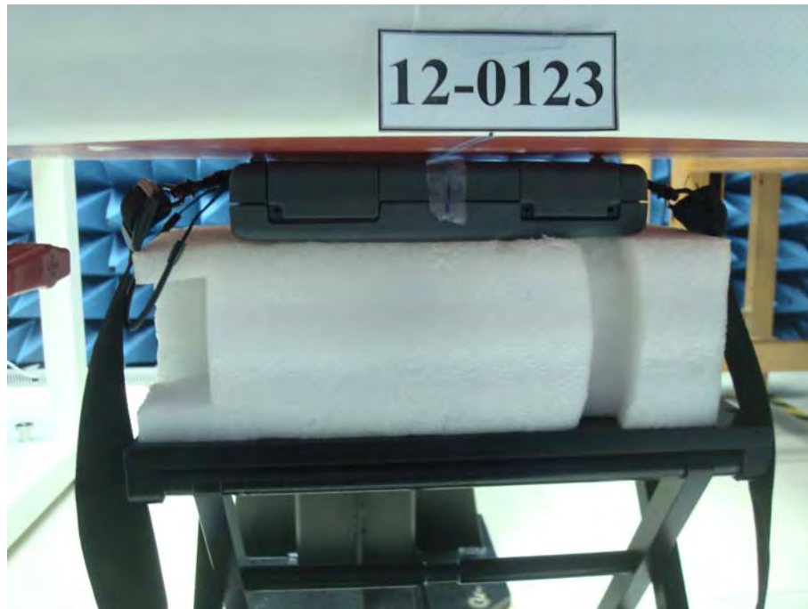
Body Setup (EUT with Internal Battery and Shoulder Strap, Back surface to phantom 0mm)
