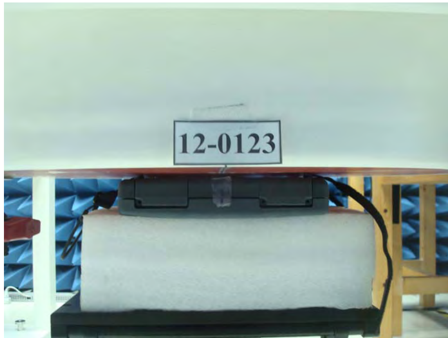
Body Setup (EUT with Internal Battery and Hand Strap, Back surface to phantom 0mm)
