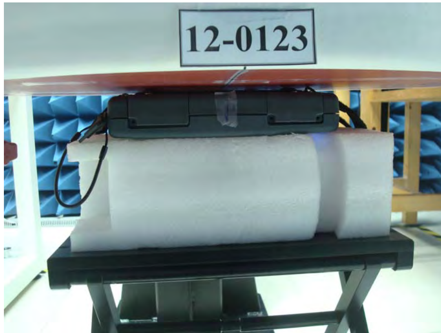
Body Setup (EUT with Thin Battery and Hand Strap, Back surface to phantom 0mm)
