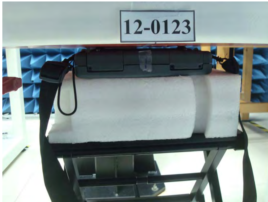
Body Setup (EUT with Thin Battery and Shoulder Strap, Back surface to phantom 0mm)
