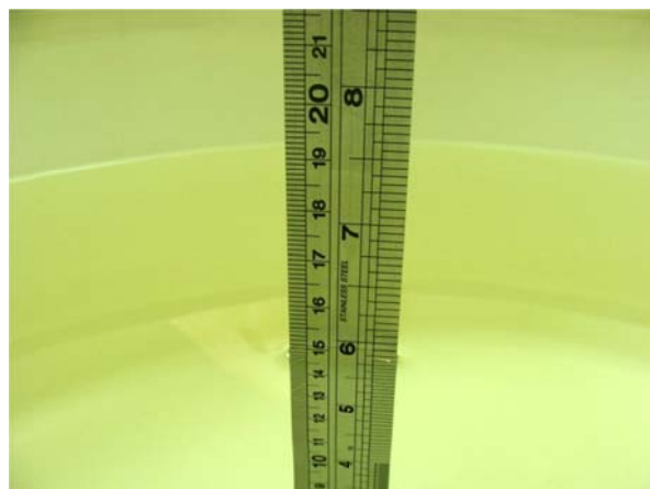
Fig 6.2 Photo of Liquid Height for Body SAR
