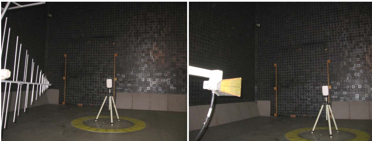
Photograph 8.1.1 Setup for radiated emission measurements
