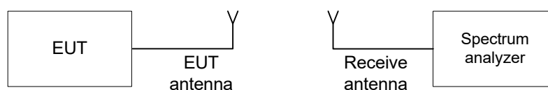
Figure 7.7.1 Band edge emission test setup
