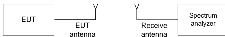
Figure 7.2.1 Occupied bandwidth test setup
