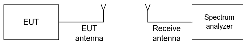
Figure 7.7.1 Band edge emission test setup
