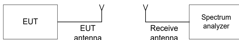
Figure 7.4.1 Average time of occupancy test setup
