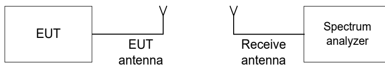
Figure 7.2.1 Carrier frequency separation test setup
