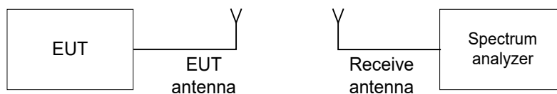
Figure 7.1.1 The 20 dB bandwidth test setup
