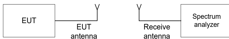
Figure 7.3.1 Hopping frequencies test setup
