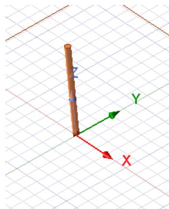
**Key features:****Frequency band: 868/914MHz****Maximum gain: 2.12dBi****Horizontal polarization****1. Antenna electrical characteristics**
