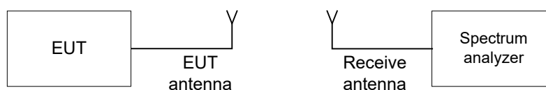
Figure 7.2.1 Carrier frequency separation test setup
