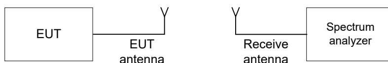
Figure 7.7.1 Band edge emission test setup
