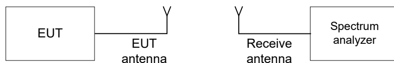
Figure 7.2.1 Carrier frequency separation test setup
