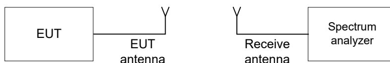
Figure 7.3.1 Hopping frequencies test setup
