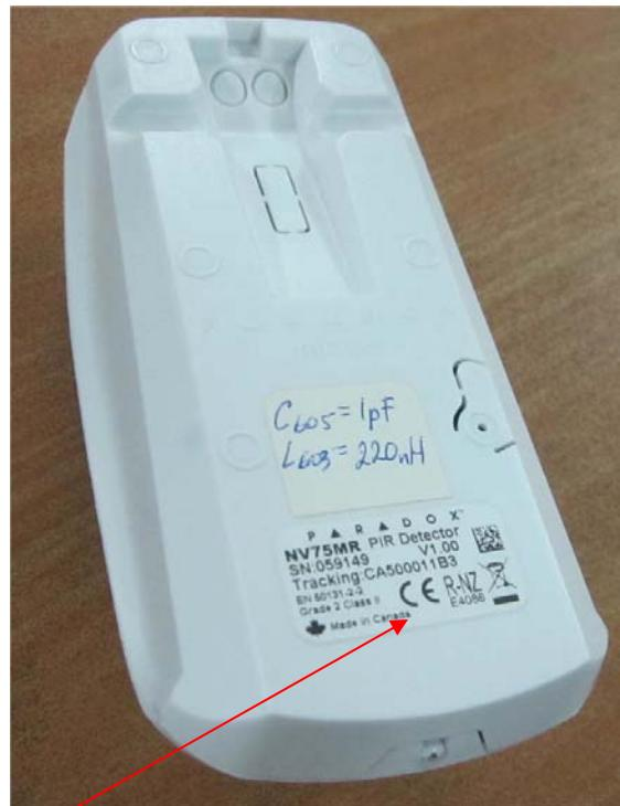
Label with **FCC ID:KDYNV75MR** and **IC:2438A-NV75MR** will be located at the rear side panel. The statement according to FCC part 15 §15.19(a)(3) is placed in User Manual, page 3 (Application exhibit User\_manual\_28739).
