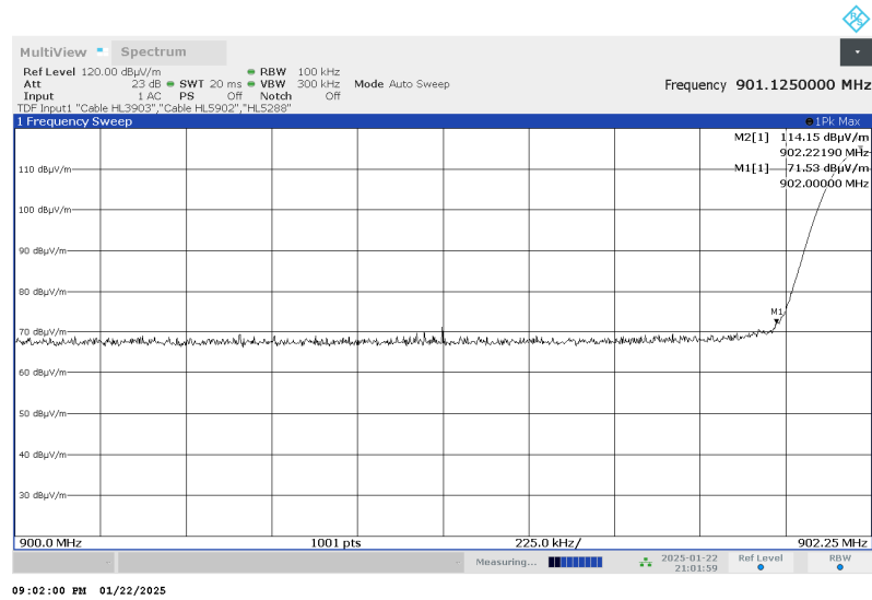
Plot 7.8.2 The highest band edge emission at high carrier frequency with hopping function disabled
