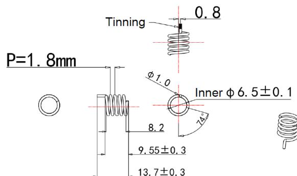
**Key features:****Frequency band: 868/914MHz****Horizontal polarization**
