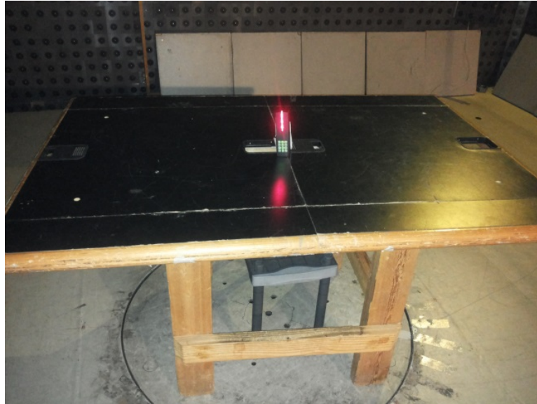
Photograph 8.2.2 Setup for radiated emission measurements, EUT close view
