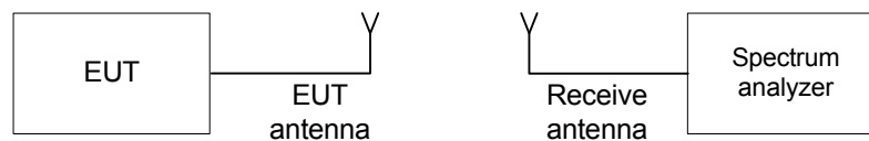
Figure 7.3.1 Occupied bandwidth test setup
