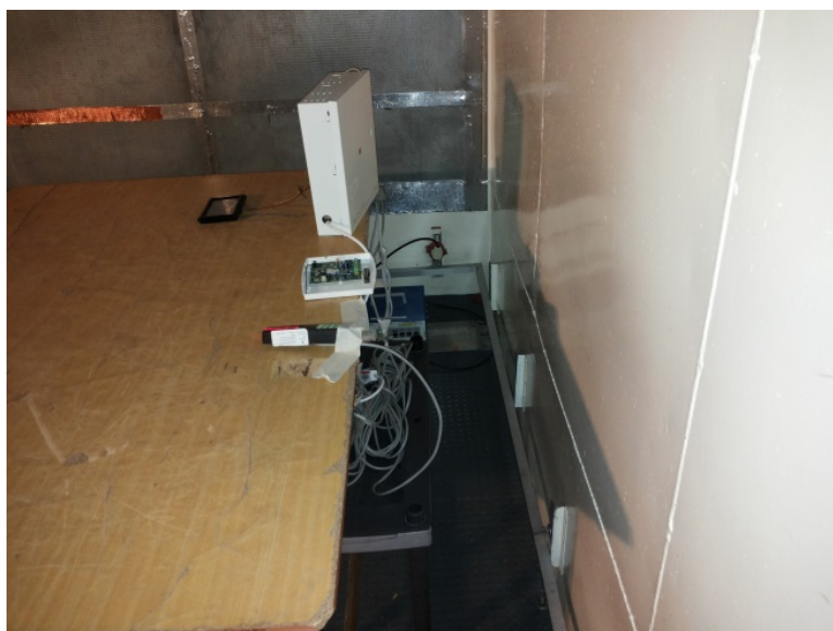
Photograph 8.1.2 Setup for conducted emission measurements
