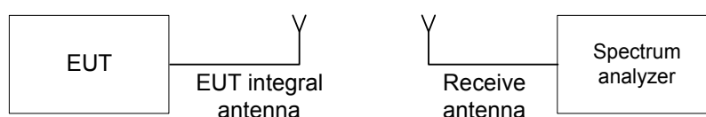
Figure 7.1.1 Setup for transmitter shut down test
