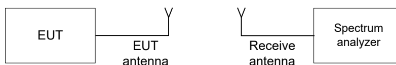
Figure 7.3.1 Hopping frequencies test setup
