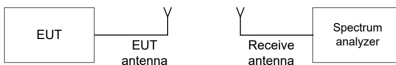
Figure 7.2.1 Carrier frequency separation test setup
