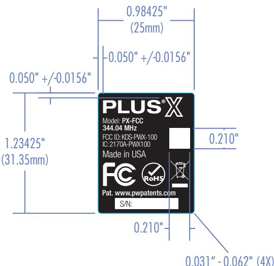
.185 Inches x .185 Inches 2D Data Matrix barcode to be centered in knocked out space which is .21 Inches x .21 Inches. 2D barcode and human readable serial number to be printed by **EPE**
