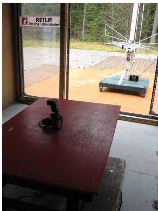
Horizontal Antenna Polarization, 30 to 1000 MHz
