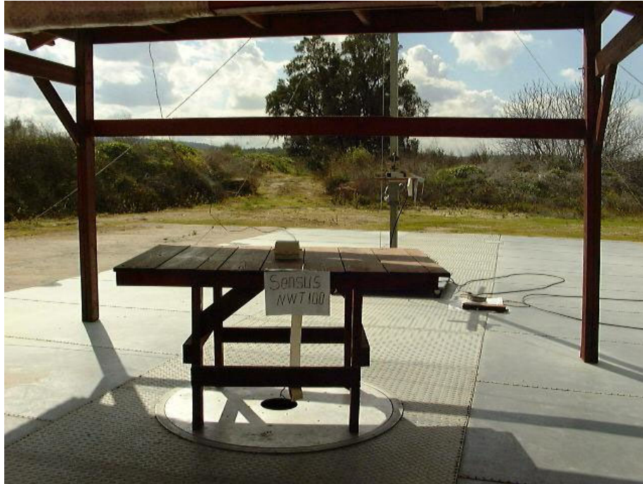
Figure 1. Spurious Radiated Emission Test Front
