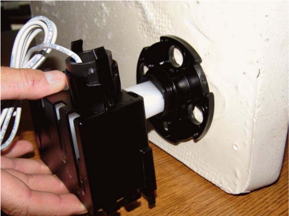
Insertion of the Endpoint into the Pit Lid Housing
