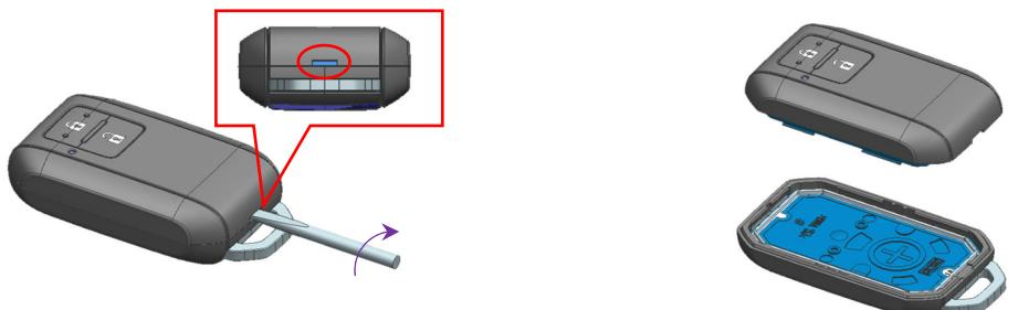
Insert a flat-blade screwdriver and twist it.
