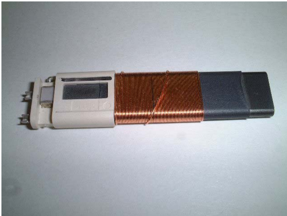
Antenna inside side A
