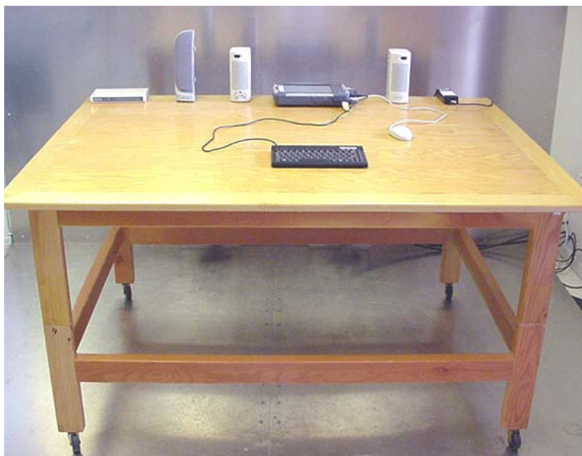
Photograph G-2 - AC Powerline Conducted Emission Configuration
