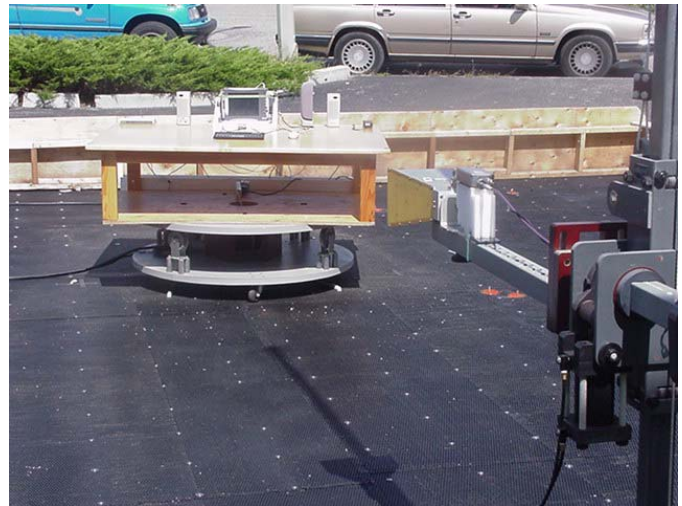
Photograph K.7-3 - Vertical 3115 Horn and LNA PCS Band Radiated Emissions 1-meter Setup
