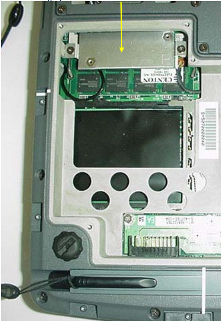
Photograph A.1-5 - Internal Bluetooth Location
