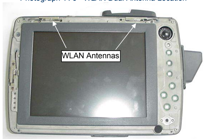
Photograph A-6 - WLAN Dual Antenna Location
