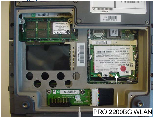
Photograph A-5 - WLAN Mini-PCI Card Location
