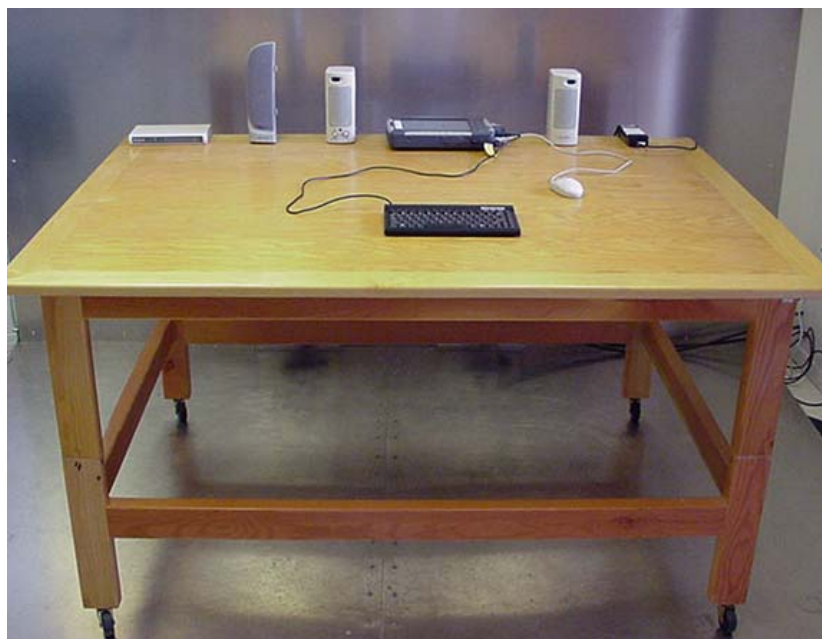
Photograph G-2 - AC Powerline Conducted Emission Configuration
