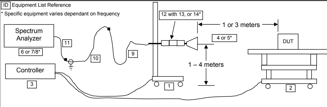
Figure K.6-2 - Signal Substitution Setup Drawing
