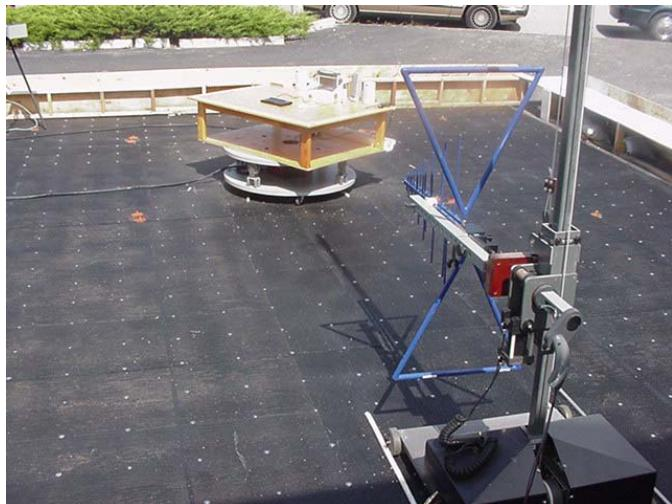
Photograph K.7-2 - Vertical 3115 Horn and LNA PCS Band Radiated Emissions 3-meter Setup
