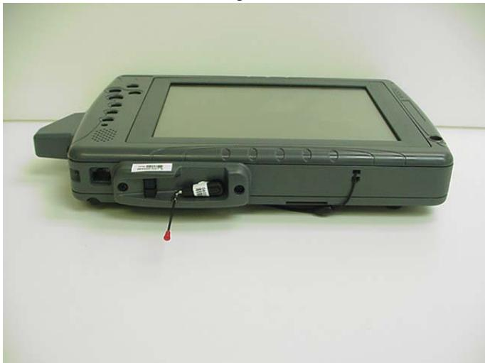
Photograph A.1-2 - Tablet PC in the worst-case PCS Configuration
