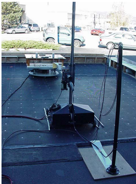
Photograph J.7-3 - Portable 3 m Horn setup
