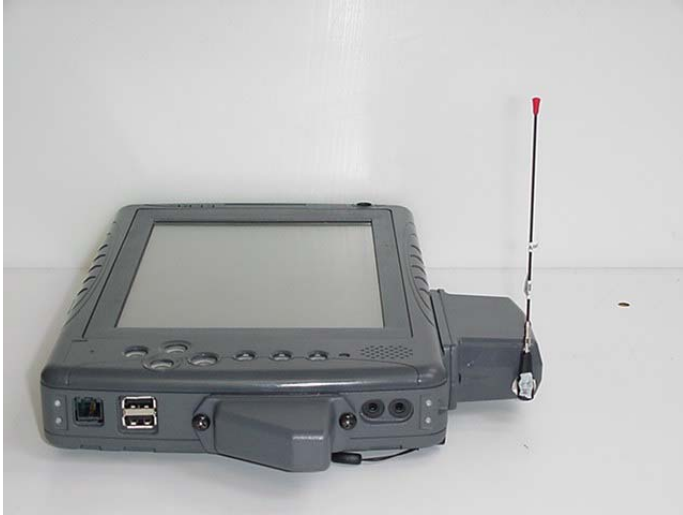
Photograph A.1-1 - Tablet PC in the worst-case Cellular Portable Configuration
