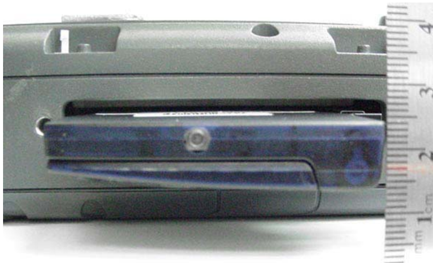
AirCard 580 Card-to-Base Distance (Broadband Hatch & Antenna Removed)
