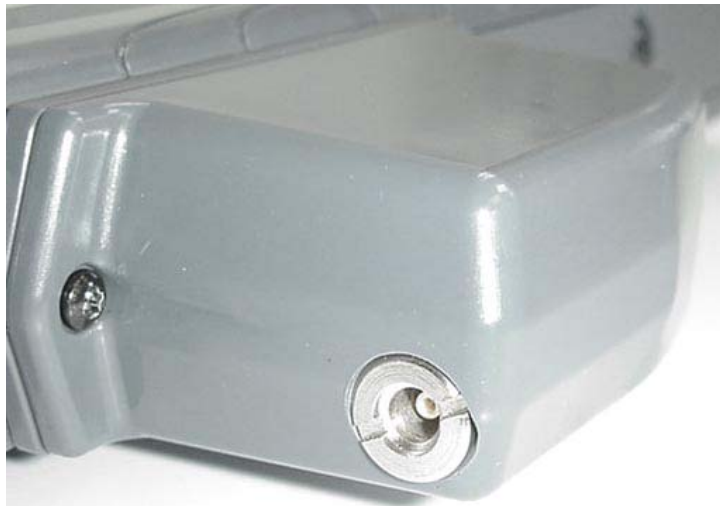
IX325 Broadband Hatch (AirCard 580 Antenna Connector)
