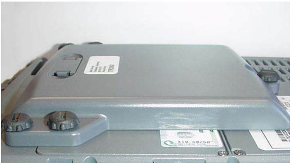
External Second Lithium-ion Battery (Model: T8S-E)
