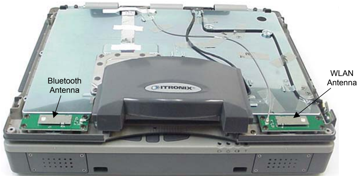
Photograph A-7 – Surface Mount Antenna Placement
