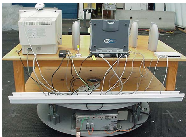
Photograph D.7-4 - Back of Radiated Emission Setup
