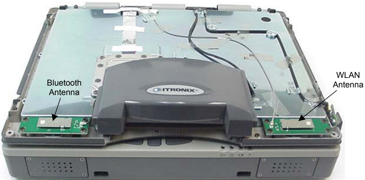
Photograph A-7 - Surface Mount Antenna Placement
