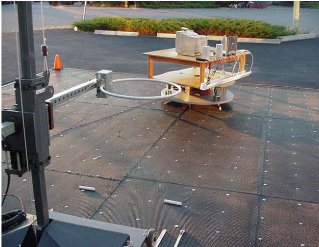
Photograph I-3 - Horizontal Polarization (30MHz - 1 GHz)
