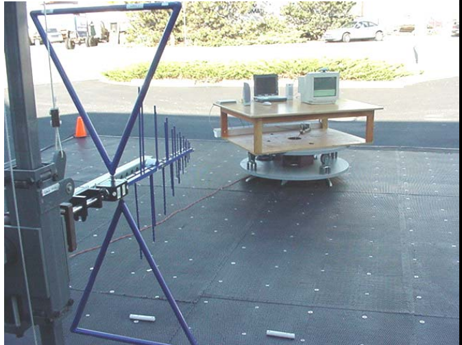
Photograph I-4 - Vertical Polarization (30MHz - 1 GHz)
