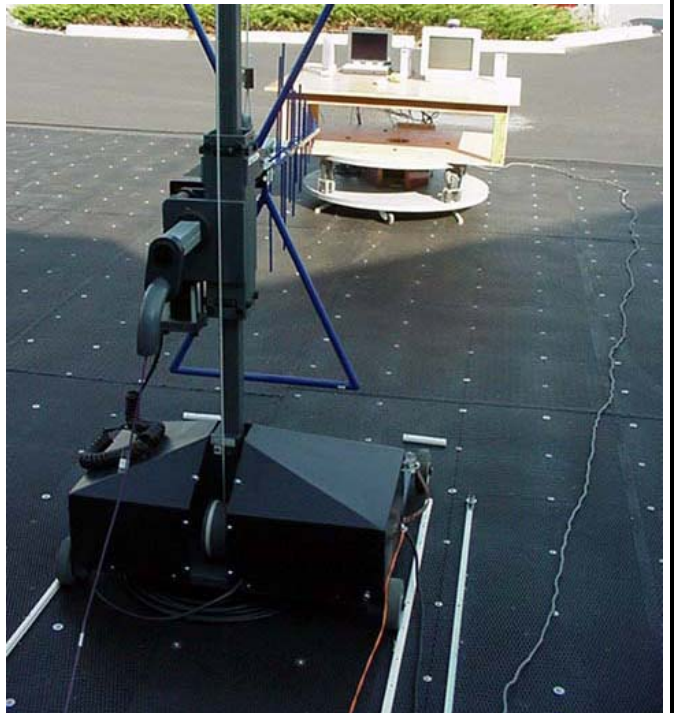
Photograph I-4 - Vertical Polarization (30MHz - 1 GHz)
