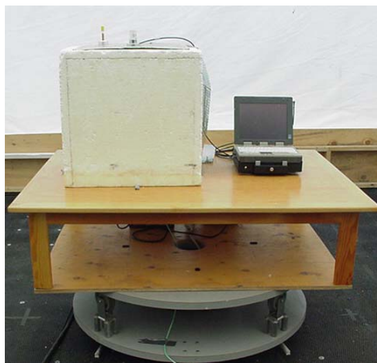
Photograph F.7-4 - Front of Radiated Emission Setup with vehicle-mount antenna and cradle
